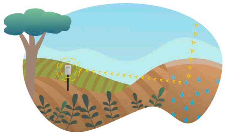
Figure 2. The Finapp probe measures the neutrons formed by the interaction between cosmic rays and water.
